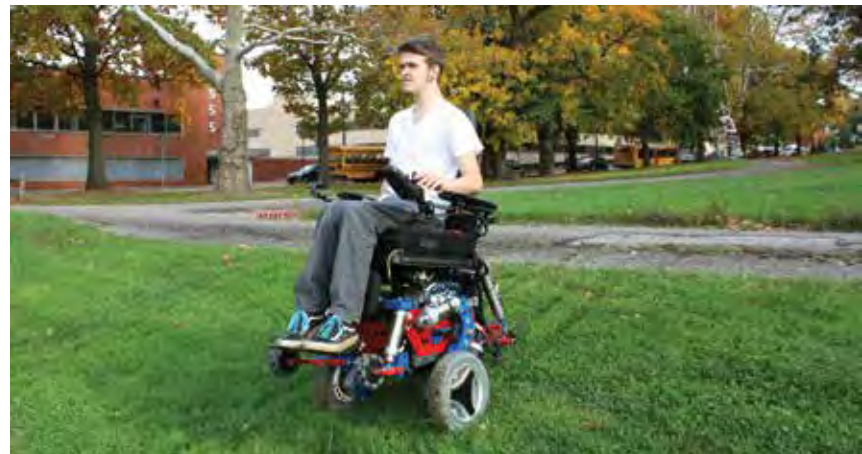
▲ Six independent, height-adjustable wheels allow MEBot to adjust to different terrains.
